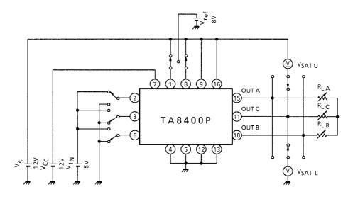
Note: Calibrate  $I_{OUT}$  to 0.4 / 1.0A by  $R_{LA}$ ,  $R_{LB}$  and  $R_{LC}$ .
