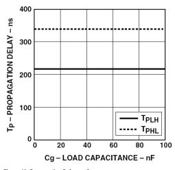
Figure 12. Propagation Delay vs. Cg.
