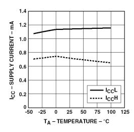
Figure 5. I<sub>CC</sub> vs. Temperature.
