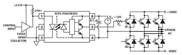
Figure 17. Recommended LED Drive and Application Circuit for ACPL-P302/W302
