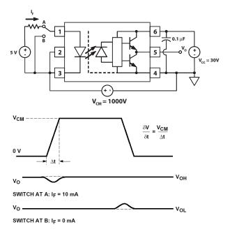
Figure 16. CMR Test Circuit and Waveforms.
