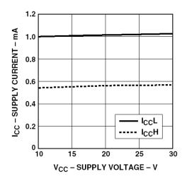
Figure 6. I<sub>CC</sub> vs. V<sub>CC</sub>.
