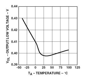
Figure 3. Vol vs. Temperature.
