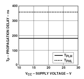
Figure 8. Propagation delay vs. V<sub>CC</sub>.
