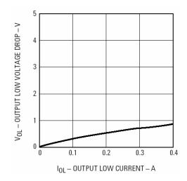
Figure 4. V<sub>OL</sub> vs. I<sub>OL</sub>.
