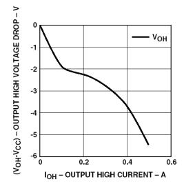
Figure 2. V<sub>OH</sub> vs. I<sub>OH</sub>.
