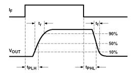
Figure 15. Propagation Delay Test Circuit and Waveforms.
