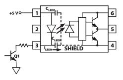
Figure 22. Not Recommended Open Collector Drive Circuit.
