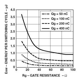
Figure 18. Energy Dissipated in the ACPL-P302/W302 and for Each IGBT Switching Cycle.
