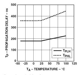
Figure 10. Propagation Delay vs. Temperature.
