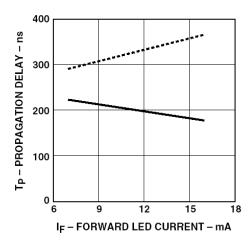
Figure 9. Propagation Delay vs. IF.
