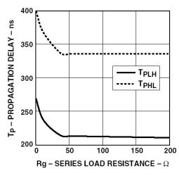
Figure 11. Propagation Delay vs. Rg.
