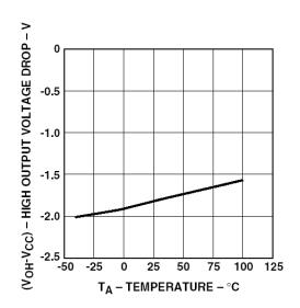
Figure 1. V<sub>OH</sub> vs. Temperature.
