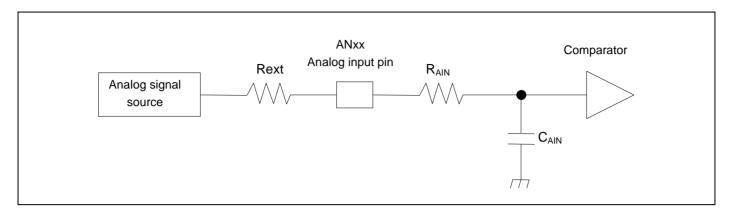
(Equation 1) Ts  $\geq$  ( R<sub>AIN</sub> + Rext )  $\times$  C<sub>AIN</sub>  $\times$  9
