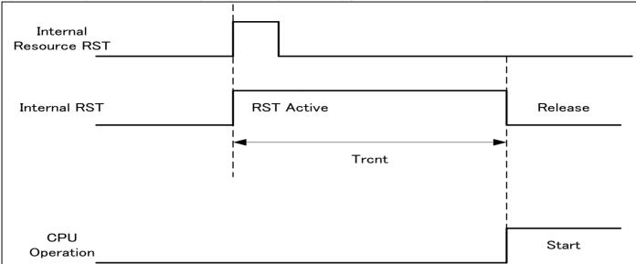
[1]: Internal resource reset is not included in return factor by the kind of Low-Power consumption mode.
