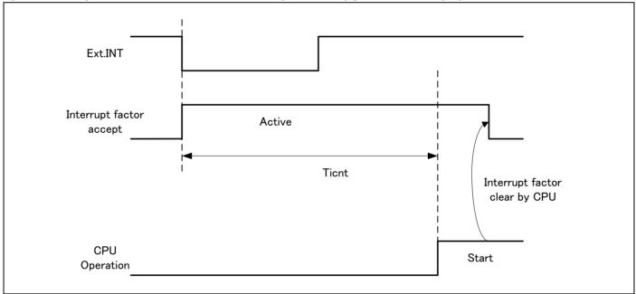
[1]: External interrupt is set to detecting fall edge.
