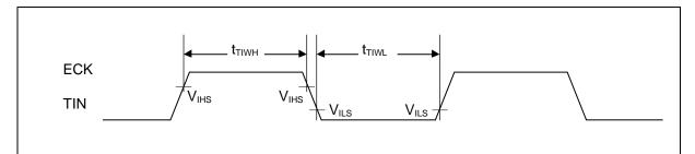
• Trigger input timing
