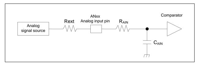
(Equation 1) Ts  $\geq$  ( R<sub>AIN</sub> + Rext ) × C<sub>AIN</sub> × 9
