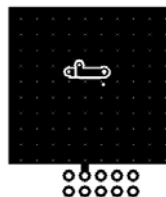
a. 60^\circ\text{C}/\text{W} when mounted on a 1 in 2 pad of 2 oz copper
