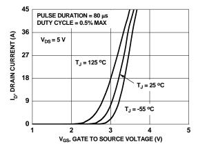
Figure 5. Transfer Characteristics
