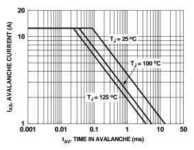
Figure 9. Unclamped Inductive Switching Capability
