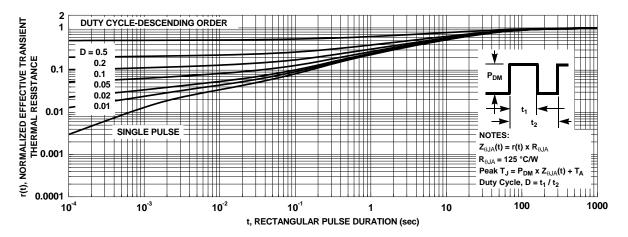
Figure 12. Junction-to-Ambient Transient Thermal Response Curve
