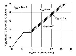
Figure 7. Gate Charge Characteristics
