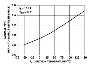
Figure 3. Normalized On-Resistance vs Junction Temperature
