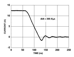
Figure 13. SyncFET body diode reverse recovery characteristic
