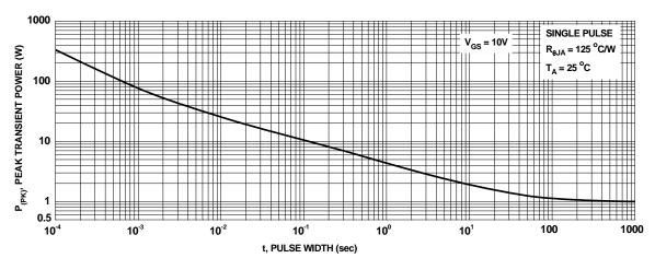
Figure 11. Single Pulse Maximum Power Dissipation
