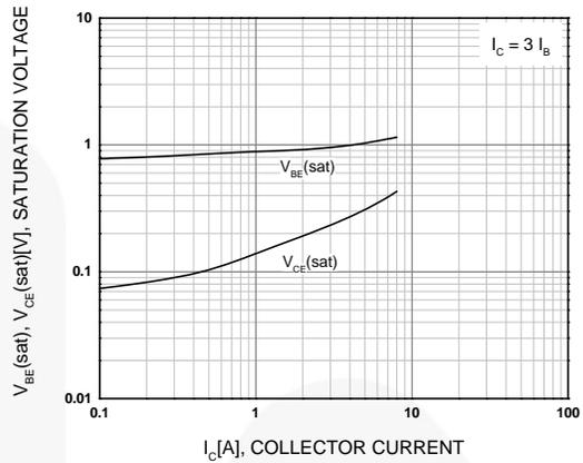
Figure 2. Saturation Voltage
