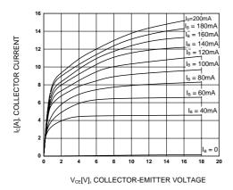
Figure 1. Static Characteristic
