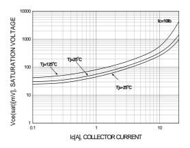
Figure 4. Collector-Emitter Saturation Voltage
