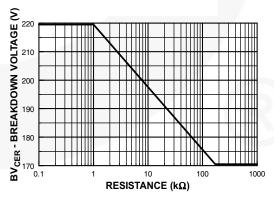
Figure 6. Collector-Emitter Breakdown Voltage with Resistance Between Emitter-Base
