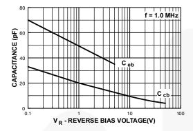
Figure 7. Input and Output Capacitance vs. Reverse Voltage
