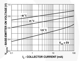
Figure 4. Base-Emitter On Voltage vs.Collector Current
