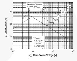
Figure 9-2. Maximum Safe Operating Area for FQPF5N60C
