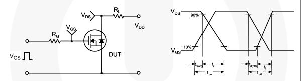
Figure 13. Resistive Switching Test Circuit & Waveforms
