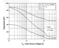
Figure 5. Capacitance Characteristics
