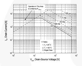
Figure 9-1. Maximum Safe Operating Area for FQP5N60C
