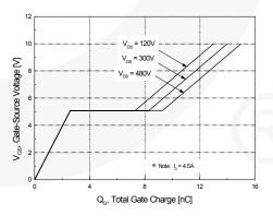
Figure 6. Gate Charge Characteristics
