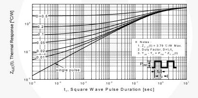
Figure 11-2. Transient Thermal Response Curve for FQPF5N60C
