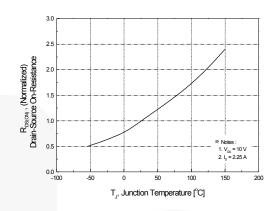
Figure 8. On-Resistance Variation vs Temperature
