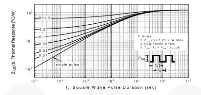
Figure 11-1. Transient Thermal Response Curve for FQP5N60C
