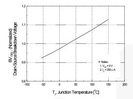
Figure 7. Breakdown Voltage Variation vs Temperature
