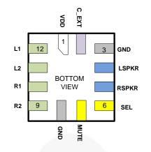
Figure 3. Pin Assignment (Bottom View)
