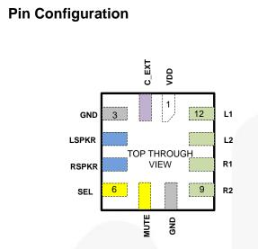
Figure 2. Pin Assignment (Top Through View)
