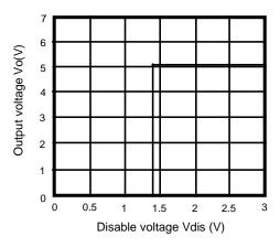
Figure 3. Output Voltage vs. Disable Voltage
