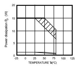
Figure 7. Power Dissipation vs. Temperature(Ta)
