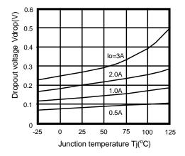
Figure 6. Dropout Voltage vs. Junction Temperature
