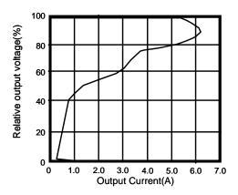
Figure 8. Overcurrent Protection Characteristics (Typical Value)
