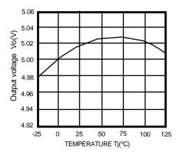
Figure 4. Output Voltage vs. Temperature(Tj)
