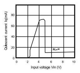
Figure 2. Quiescent Current vs. Input Voltage
