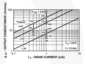
Figure 10. Output Conductance vs. Drain Current
