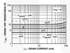
Figure 9. On Resistance vs. Drain Current
