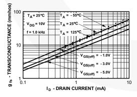
Figure 11. Transconductance vs. Drain Current
