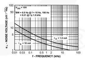
Figure 6. Noise Voltage vs. Frequency
