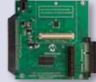
MRF24J40MA PICtail Plus 2.4 GHz RF Card (AC164134)
