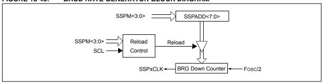
ote: Values of 0x00, 0x01 and 0x02 are not valid for SSPADD when used as a Baud Rate Generator for I<sup>2</sup>C. This is an implementation limitation.
