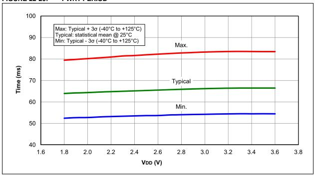
FIGURE 22-21: FVR STABILIZATION PERIOD
