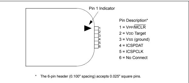
For additional interface recommendations, refer to your specific device programmer manual prior to PCB design.
