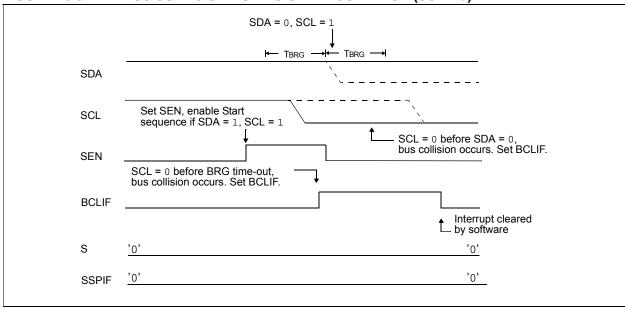
FIGURE 18-35: BRG RESET DUE TO SDA ARBITRATION DURING START CONDITION
