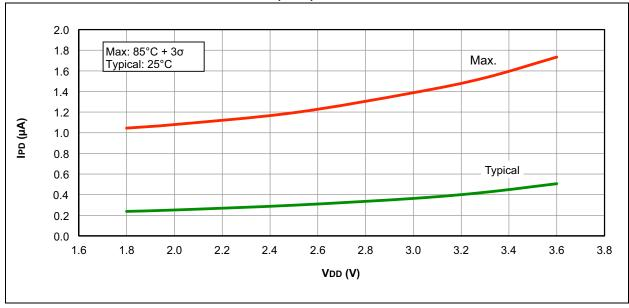
FIGURE 22-12: IPD, FIXED VOLTAGE REFERENCE (FVR)
