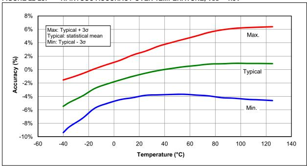
FIGURE 22-24: HFINTOSC ACCURACY OVER TEMPERATURE, 2.3V ≤ VDD ≤ 3.6V
