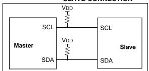
The Acknowledge bit (ACK) is an active-low signal, which holds the SDA line low to indicate to the transmitter that the slave device has received the transmitted data and is ready to receive more.
