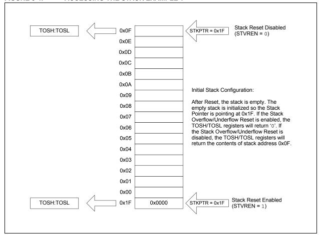
FIGURE 3-5: **ACCESSING THE STACK EXAMPLE 2** 0x0F 0x0E 0x0D 0x0C 0x0B 0x0A 0x09 This figure shows the stack configuration after the first  $\mathtt{CALL}$  or a single interrupt. 80x0 If a RETURN instruction is executed, the return address will be placed in the 0x07 Program Counter and the Stack Pointer decremented to the empty state (0x1F). 0x06 0x05 0x04 0x03 0x02 0x01 TOSH:TOSL 0x00 Return Address STKPTR = 0x00
