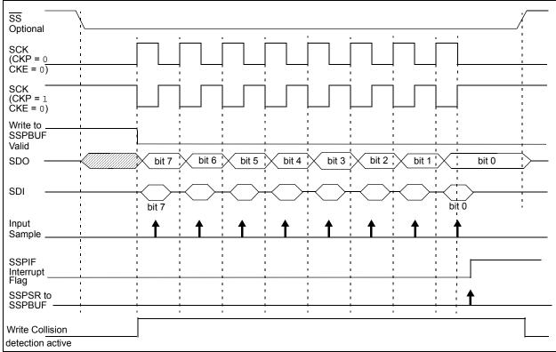
FIGURE 18-10: SPI MODE WAVEFORM (SLAVE MODE WITH CKE = 1)
