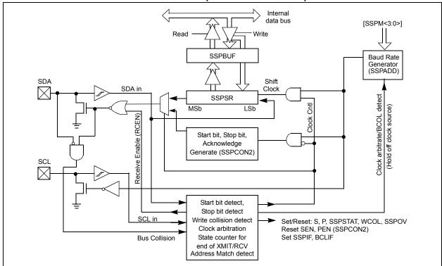
FIGURE 18-3: MSSP1 BLOCK DIAGRAM (I<sup>2</sup>C™ SLAVE MODE)
