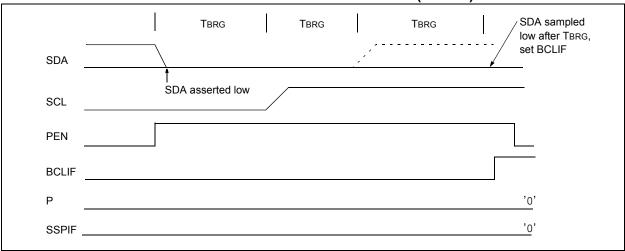
FIGURE 18-39: BUS COLLISION DURING A STOP CONDITION (CASE 2)
