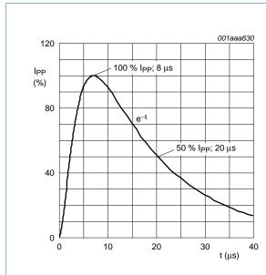
Fig 1. 8/20  $\mu s$  pulse waveform according to IEC 61000-4-5
