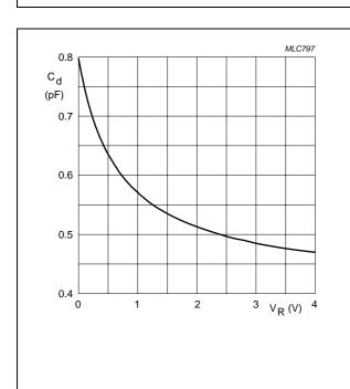
$f = 1 \text{ MHz}; T_{amb} = 25 \,^{\circ}\text{C}.$
