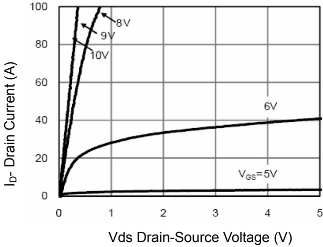
**Figure 1 Output Characteristics**
