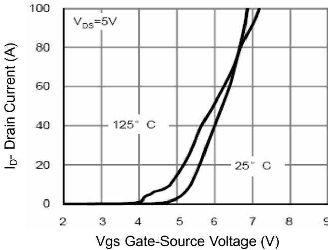
**Figure 2 Transfer Characteristics**
