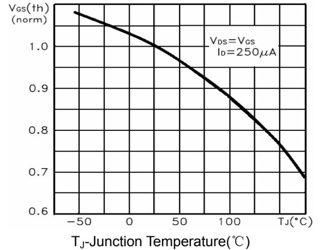
**Figure 10 V<sub>GS(th)</sub> vs Junction Temperature**
