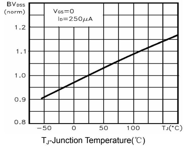
**Figure 9 BV<sub>DSS</sub> vs Junction Temperature**
