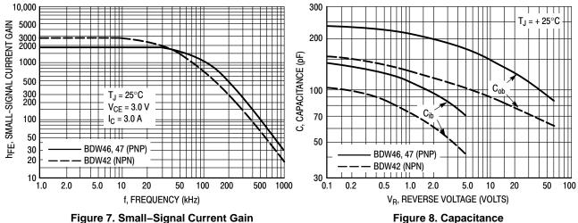
Figure 7. Small–Signal Current Gain
