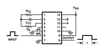
FIGURE 3. DIGITAL TIMER APPLICATION CIRCUIT
