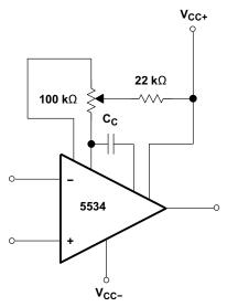
Frequency Compensation and Offset-Voltage Nulling Circuit
