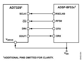
Figure 59. Interfacing the AD7329 to the ADSP-BF53x
