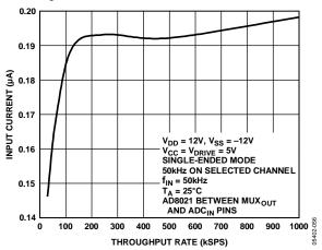
Figure 32. Input Current vs. Throughput Rate with AD8021 Between MUX<sub>OUT</sub> and ADC<sub>IN</sub>
