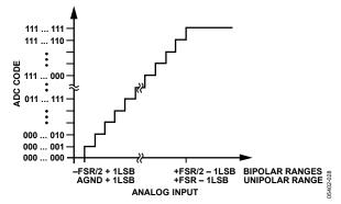
Figure 29. Straight Binary Transfer Characteristic, Bipolar Ranges
