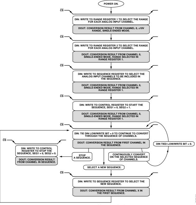
Figure 48. Programmable Sequence Flowchart
