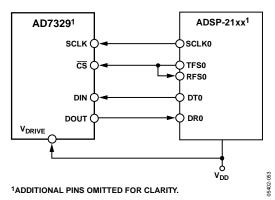
Figure 58. Interfacing the AD7329 to the ADSP-21xx
