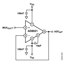
Figure 47. AD8021 Configuration Used Between MUX<sub>OUT</sub> and ADC<sub>IN</sub> Pins
