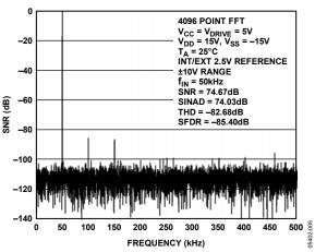
Figure 5. FFT for Single-Ended Mode
