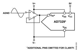
Figure 36. Single-Ended Mode Typical Connection Diagram
