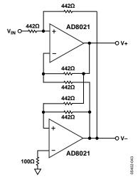
Figure 46. Single-Ended-to-Differential Configuration with the AD8021
