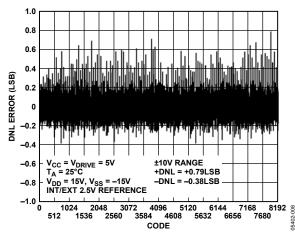
Figure 8. Typical DNL for Single-Ended Mode
