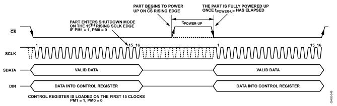
Figure 54. Entering Autoshutdown/Autostandby Mode
