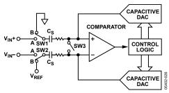
Figure 27. ADC Configuration During Conversion Phase, Differential Mode
