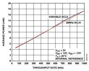
Figure 56. Power vs. Throughput Rate with 5 V Vcc
