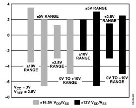
Figure 44. Pseudo Differential Input Range with  $V_{CC} = 3 V$
