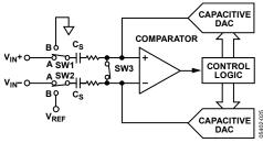
Figure 26. ADC Configuration During Acquisition Phase, Differential Mode
