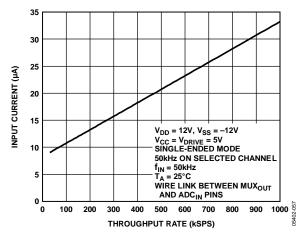
Figure 33. Input Current vs. Throughput Rate with a Wire Link Between MUX<sub>OUT</sub> and ADC<sub>IN</sub>
