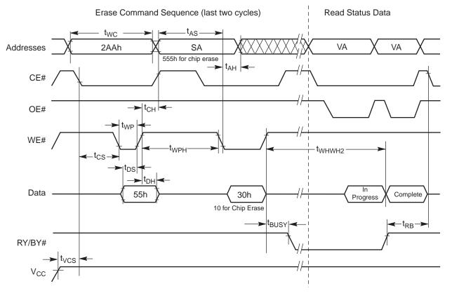
Figure 15.7 Chip/Sector Erase Operation Timings
