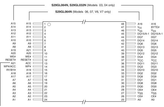
Figure 3.1 48-Pin Standard TSOP
