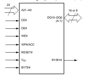
Figure 5.1 S29GL064N Logic Symbol (Models 01, 02, V1, V2)
