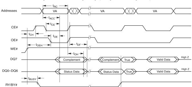
Figure 15.8 Data# Polling Timings (During Embedded Algorithms)
