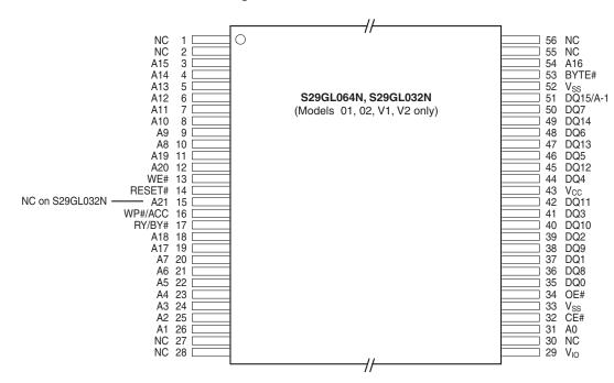
Figure 3.2 56-Pin Standard TSOP
