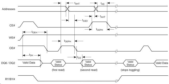
Figure 15.9 Toggle Bit Timings (During Embedded Algorithms)
