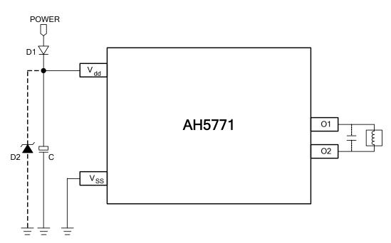
Note: D2 (Zenor Diode) and Capacitor C are for power stabilization, D2 is recommended to be 18Vz (option), C is recommended to 0.1uF ~1uF (E-Cap). D1 (reverse Diode) is for reverse voltage protection.
