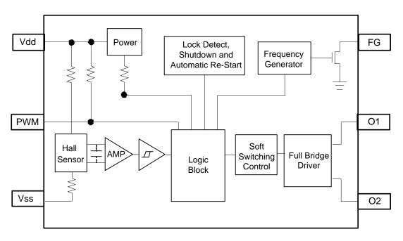
Notes: 3. The AH5795 has an open-drain tachometer FG output that follows the magnetic change frequency. Typically a pull-up resistor of 10KΩ is recommended from FG pin to the supply voltage.
