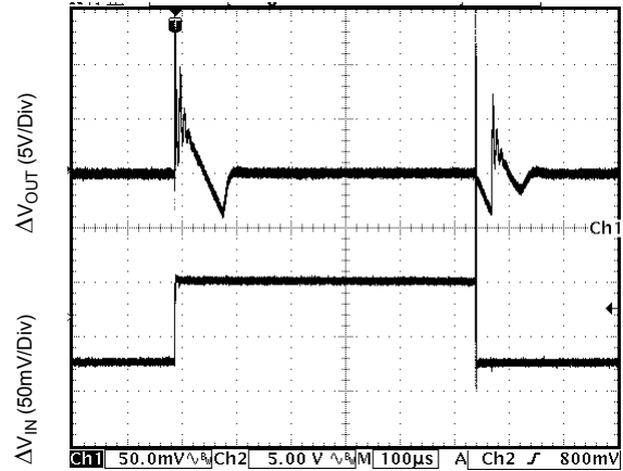
Figure 25. Line Transient Response
