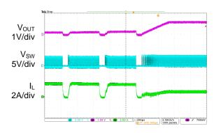
**Short Circuit Protection Recovery (Iout=1A)**
