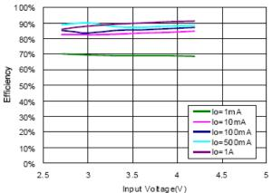
Efficiency vs Input Voltage (Vo=15V)
