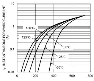
$V_{\rm F}$ , INSTANTANEOUS FORWARD VOLTAGE (mV) Figure 1. Typical Forward Characteristics
