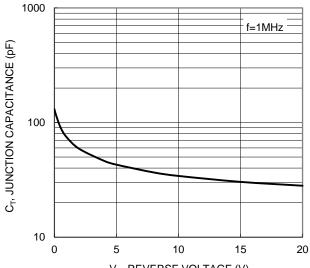
$V_{R}$ , REVERSE VOLTAGE (V) Figure 3. Typical Junction Capacitance
