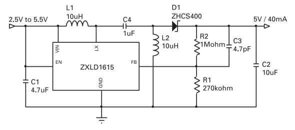
1 Cell Li-Ion to 5V Sepic Converter
