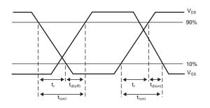
Switching time waveforms
