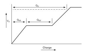
Basic gate charge waveform
