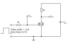
Switching time test circuit
