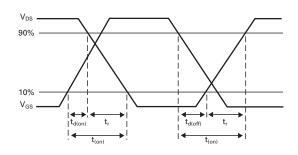
Switching time waveforms
