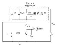
Gate charge test circuit
