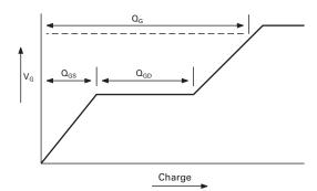
Basic gate charge waveform
