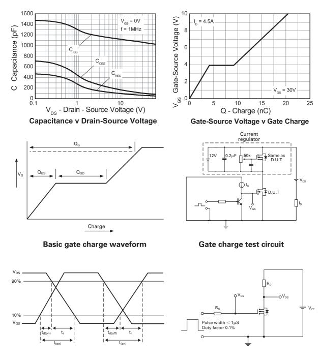
Switching time waveforms
