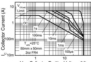
V<sub>CE</sub> Collector-Emitter Voltage (V) **Safe Operating Area**
