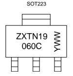
ZXTN19 060C = Product Type Marking Code YWW = Date Code Marking Y or  $\overline{Y}$  = Last Digit of Year (ex: 5= 2015) WW or  $\overline{W}W$  = Week Code (01~53)
