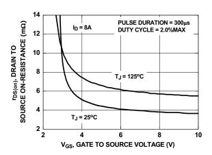
Figure 15. On-Resistance vs Gate to Source Voltage
