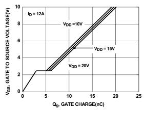
Figure 7. Gate Charge Characteristics
