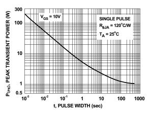
Figure 10. Single Pulse Maximum Power Dissipation
