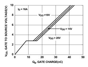
Figure 18. Gate Charge Characteristics
