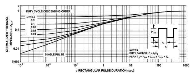
Figure 11. Transient Thermal Response Curve
