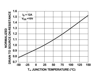
Figure 3. Normalized On-Resistance vs Junction Temperature
