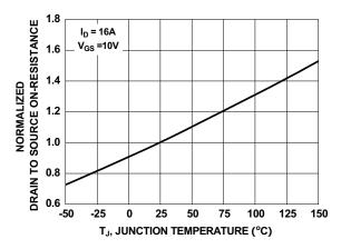
Figure 14. Normalized On-Resistance vs Junction Temperature
