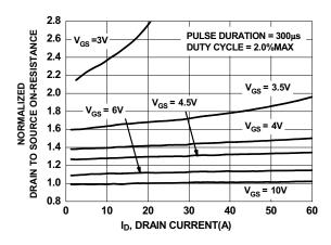
Figure 13. Normalized on-Resistance vS Drain Current and Gate Voltage
