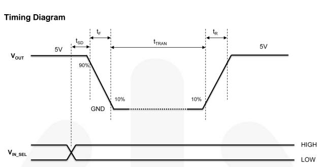
Figure 6. Transition Delay ( $V_{IN}=V_{BUS}=5~V$ )
