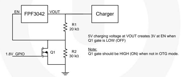
Figure 2. Example Circuit for OTG Operation with Low-Voltage GPIO
