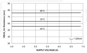
Figure 13.V<sub>IN</sub> On Resistance (mΩ) vs. Supply Voltage Figure 14.V<sub>BUS</sub> On Resistance (mΩ) vs. Supply Voltage
