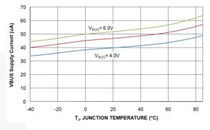
Figure 7. VIN Quiescent Current (Iq) vs. Temperature Figure 8. VBUS Quiescent Current (Iq) vs. Temperature
