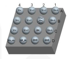
Figure 5. Pin Assignment (Bottom View)
