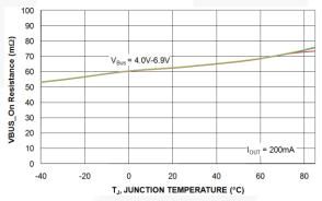
Figure 11. V<sub>IN</sub> On Resistance (mΩ) vs. Temperature
