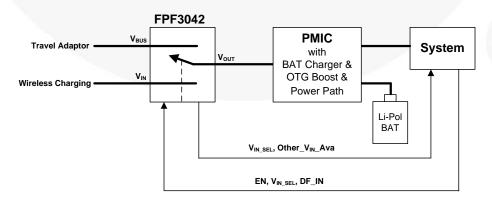
Figure 31.Input Power Selector for Wireless Charging System
