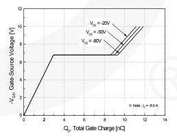
Figure 6. Gate Charge Characteristics
