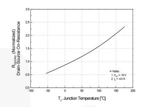
Figure 8. On-Resistance Variation vs. Temperature
