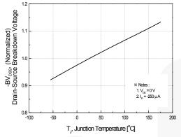
Figure 7. Breakdown Voltage Variation vs. Temperature
