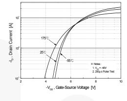
Figure 2. Transfer Characteristics
