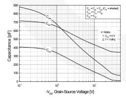
Figure 5. Capacitance Characteristics
