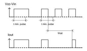
Figure 3 - Active clamp waveforms
