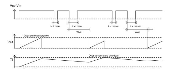
Figure 5 - Protection Timing Diagrams
