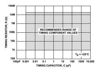
FIGURE 8. RECOMMENDED RANGE OF TIMING
