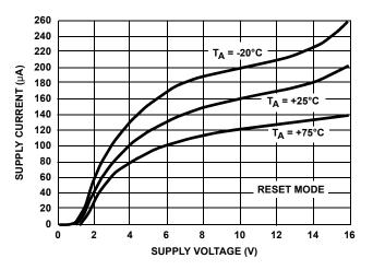
FIGURE 7. SUPPLY CURRENT vs SUPPLY VOLTAGE
