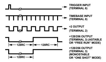
FIGURE 1. TIMING DIAGRAMS OF OUTPUT WAVEFORMS
