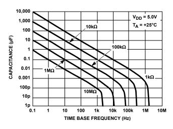
FIGURE 9. TIMEBASE FREE RUNNING FREQUENCY vs R AND C
