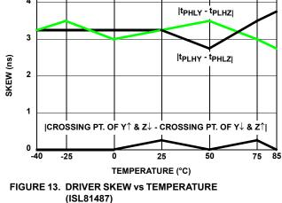
Typical Performance Curves V<sub>CC</sub> = 5V, T<sub>A</sub> = 25°C, ISL8487, ISL81483 and ISL81487; Unless Otherwise Specified (Continued)
