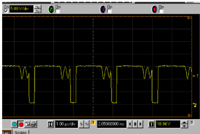
FIGURE 7. BOOST SWITCH NODE AT 100mA (PARTIAL DISCONTINUOUS)
