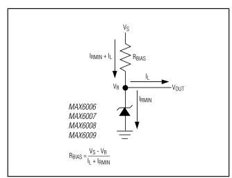
Figure 1. Typical Application Circuit
