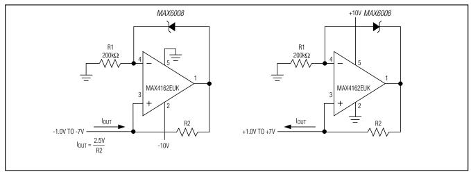
Figure 2. Precision 1µA to 1mA Current Sources
