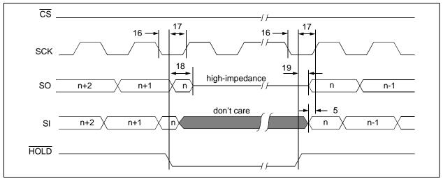
FIGURE 1-2: SERIAL INPUT TIMING
