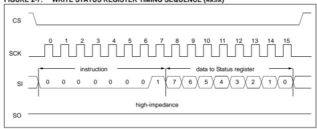
**Note:** An internal write cycle (Twc) is initiated on the rising edge of  $\overline{CS}$  after a valid write Status Register sequence.
