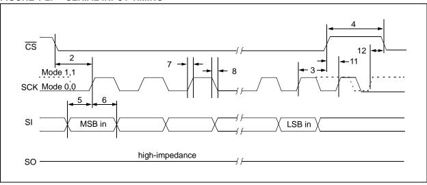
FIGURE 1-3: SERIAL OUTPUT TIMING
