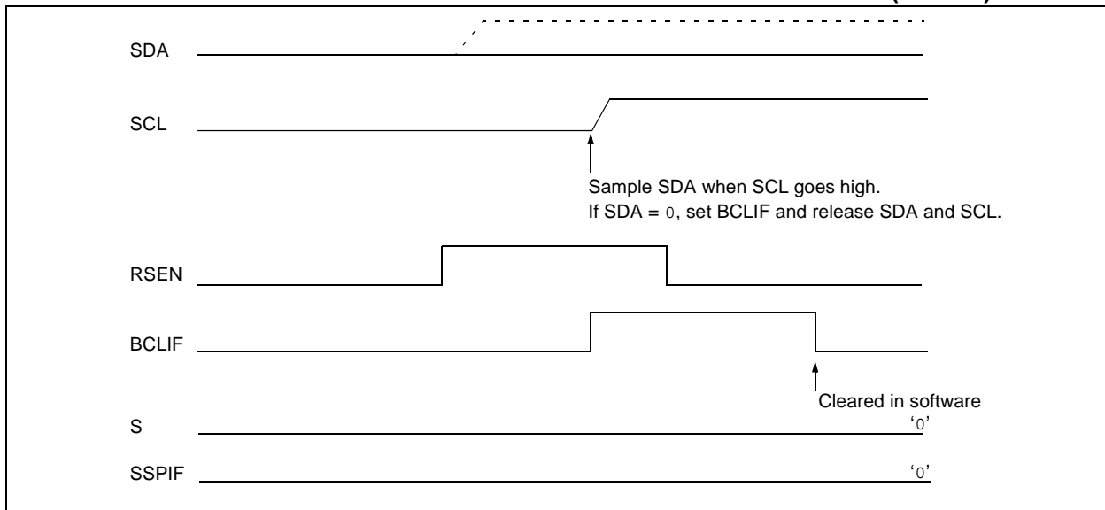
FIGURE 17-29: BUS COLLISION DURING A REPEATED START CONDITION (CASE 1)
