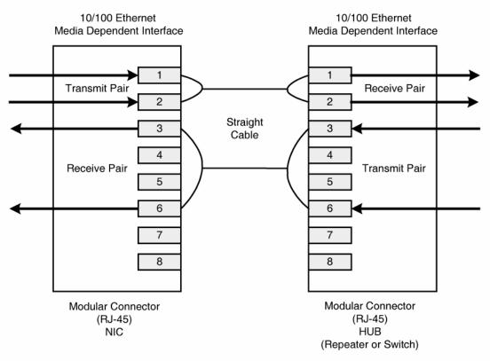
Figure 1. Typical Straight Cable Connection
