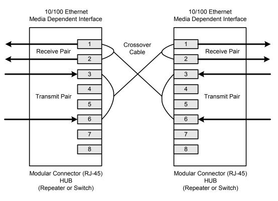
Figure 2. Typical Crossover Cable Connection
