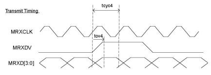
Figure 21. PHY Mode MII Timing – Data Transmitted to MII
