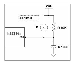
Figure 32. Recommended Reset Circuit
