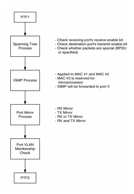
Figure 5. Destination Address Resolution Flow Chart, Stage 2
