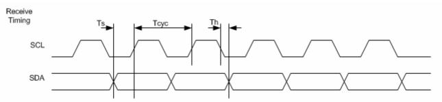
Figure 24. I2C Input Timing
