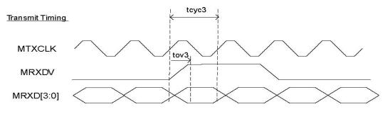
Figure 19. MAC Mode MII Timing – Data Transmitted to MII
