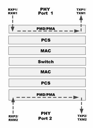
Figure 15. Near-end (Remote) Loopback Path
