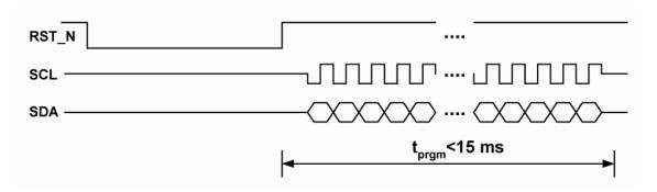
Figure 9. EEPROM Configuration Timing Diagram
