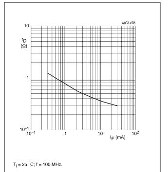
Fig.3 Diode forward resistance as a function of forward current; typical values.
