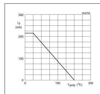
Device mounted on an FR4 printed-circuit board.
