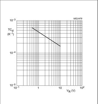
Fig.4 Temperature coefficient of diode capacitance as a function of reverse voltage; typical values.
