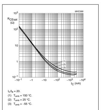
Fig.7 Equivalent on-resistance as a function of collector current; typical values.
