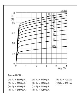
Fig.13 Collector current as a function of collector-emitter voltage; typical values.
