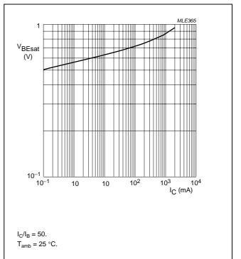
Fig.12 Base-emitter saturation voltage as a function of collector current; typical values.
