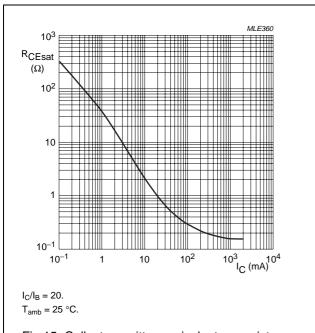
Fig.15 Collector-emitter equivalent on-resistance as a function of collector current; typical values.
